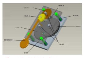
Figure 2: Pro-E Model for Gear Arrangement
